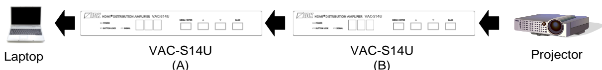
[Fig. 8.4] Reading EDID in cascade connection
