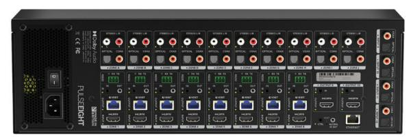
Made in partnership with Binary, the Pulse-Eight neo:X+ Video & Audio Matrix has it all - with both audio and video inputs and video and audio outputs. Featuring 8 HDMI inputs, 8 HDBaseT Outputs and 2 HDMI outputs alongside 10 audio output zones (with the options of Stereo L/R, Optical and Digital Coax) and 4 audio inputs (with the option of Optical and Digital Coax).
