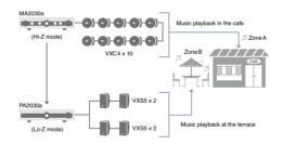
\* One DCP1V4S unit can be connected to an MA2030a. A total of two DCP units (DCP1V4S, DCP4S, DCP4V4S) can be connected to the MA2120 and PA2120.
